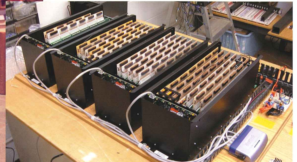
Left: The ICS-4000™ installed in a console Right: The ICS-4000™ chamber "cages" being tested in the lab.
